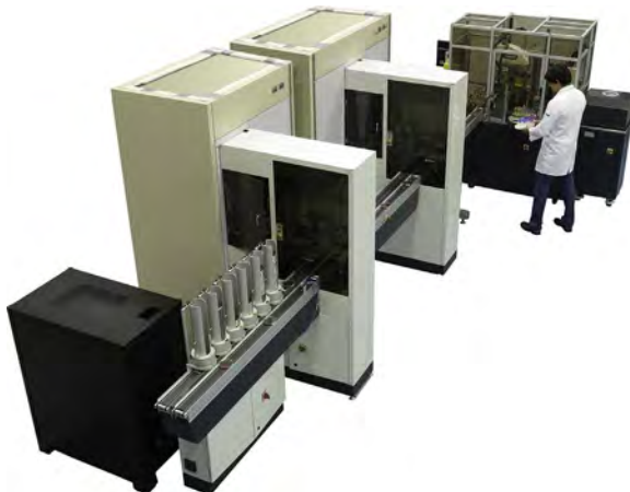
Fig. 16. WASPLab. Consists of WASP plating system, track, and incubator with digital camera. (Courtesy of Copan Diagnostics, Murrieta, CA; with permission.)
