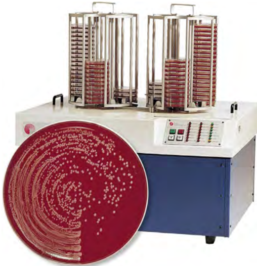
Fig. 5. Isoplater. The Isoplater is a first-generation semiautomated streak-only plating instrument. (Courtesy of Vista Technology Inc, Edmonton, Alberta Canada; with permission.)
