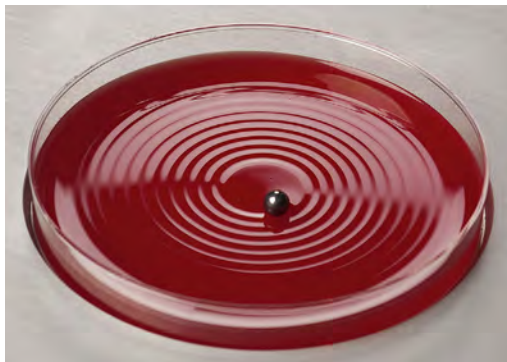
Fig. 9. Petri dish streaked with magnetic bead technology using the Inocula. (Courtesy of Becton Dickinson, Franklin Lakes, NJ; with permission.)
