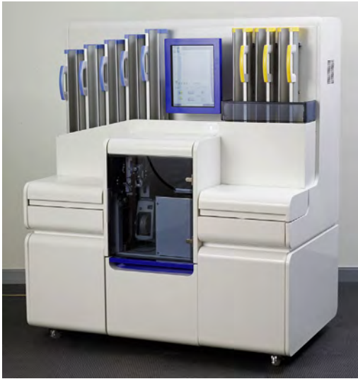
Fig. 13. PREVI Isola. The instrument accommodates 150 plates and 5 different types of media at once. (Courtesy of bioMérieux SA, Marcy l'Etoile, France.)
