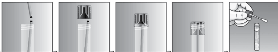
Fig 2. Capture of broken swab applicator stick by MSwab™ tube cap
