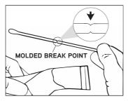
The molded breaking point is present and detectable as a narrowing of the stick.
