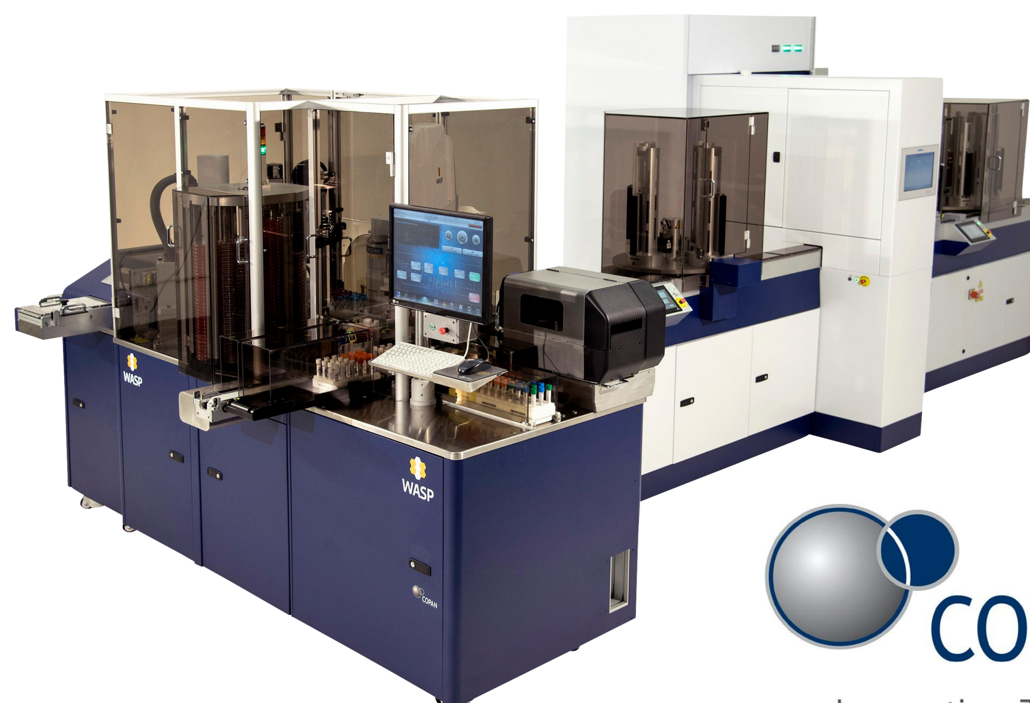
Figure 1. The WASPLab - Total Laboratory Automation system consisting of the WASP (Walk Away Specimen Processor) plating instrument, track for moving petri dishes, and a smart incubator with a 27-megapixel camera for imaging analysis.
