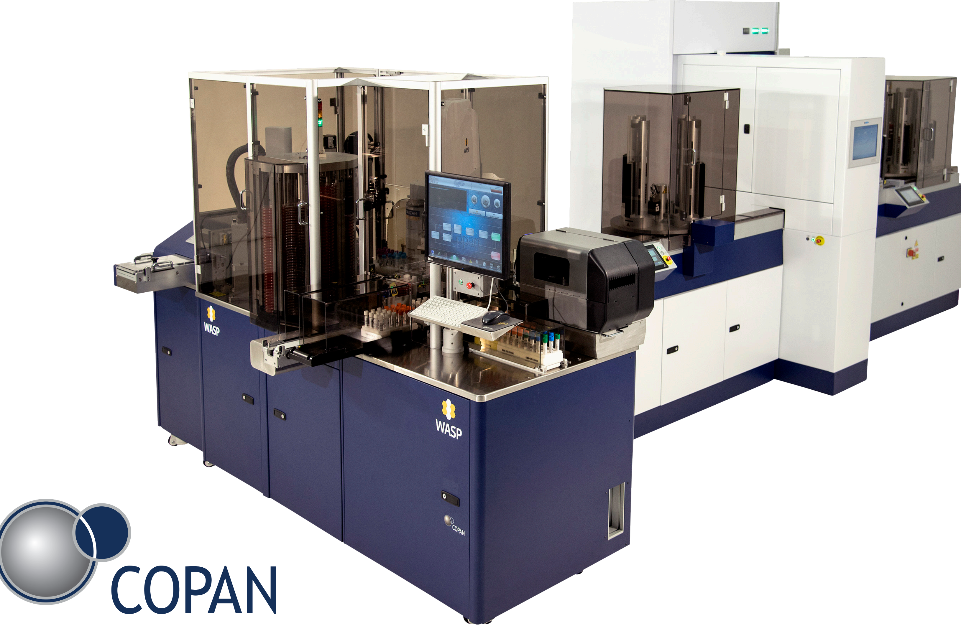
Figure 1. The WASPLab - Total Laboratory Automation system consisting of the WASP (Walk Away Specimen Processor) plating instrument, track for moving petri dishes, and a smart incubator with a 27-megapixel camera for imaging analysis.
