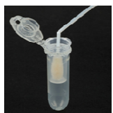
Image 2: Nylon flocked swab preparation in an NAO™.
