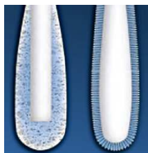
Image 2: Illustrated cross sections of cotton (left) and nylon flocked (right) swabs.
