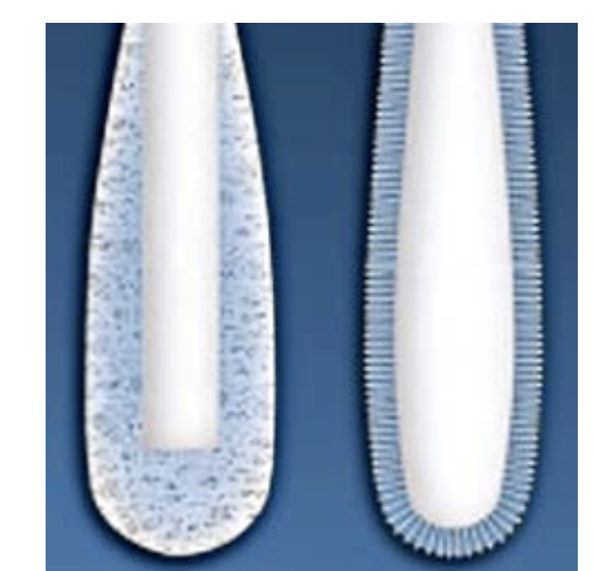
Image 6: Illustrated cross sections; Cotton (left) and Nylon (right).
